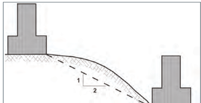
Figure 5: Footings should step at no more than 1 vertical to 2 horizontal
